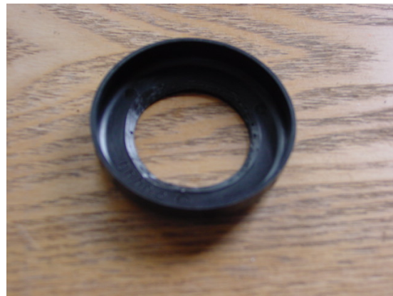
Plastic Dust Cap adapted to allow metal to metal fit of C Ring adjuster
