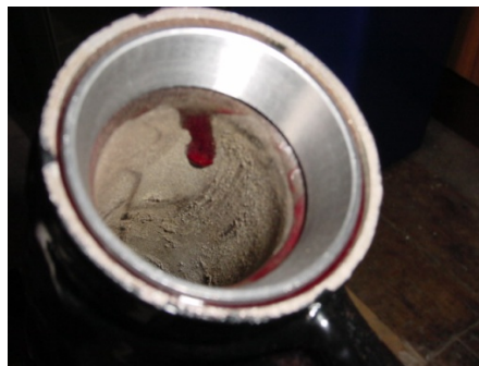
Greased Upper Bearing in place
