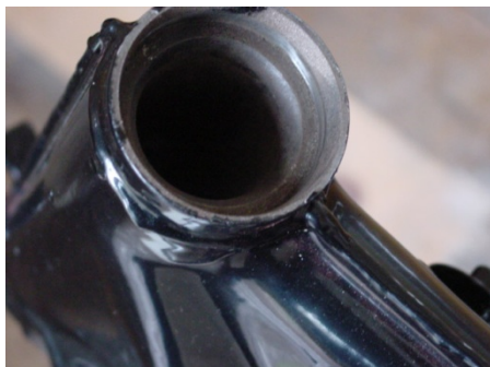
Lower Bearing installed
